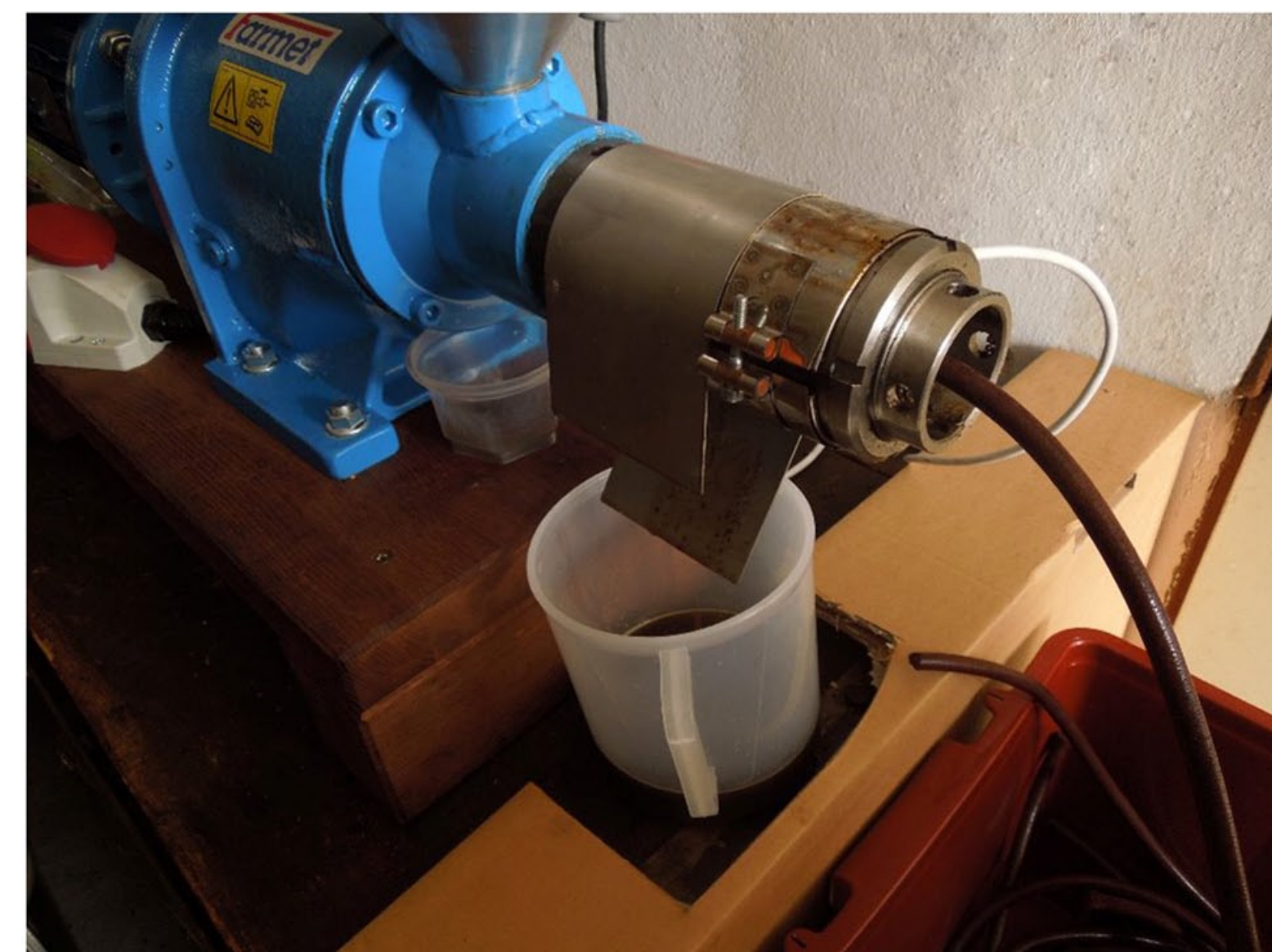
Pressing oil from the seeds using a screw press (Farmet UNO FM 3F)
